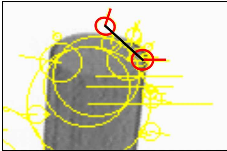
Figure 8: A sample geometric-SIFT grouping representations (two SIFT keys related by angle of the center-center orientation axis).
